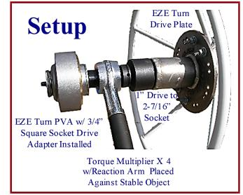
The mechanical advantage in the use of your torque multiplier is derived from the planetary transmission within the gear head of the tool. With the torque multiplier reaction bar in a fixed position against a stationery object the EZE Turn Portable Valve Actuator drives the socket and drive plate which see forces equaling the ratio 4X the output of the PVA. Due to frictional losses in the gear train a torque loss factor of 10 to 20% should be anticipated.
