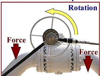
CAUTION: DO NOT EXCEED THE RATED CAPACITY FOR THE TORQUE MULTIPLIER. EXCESSIVE FORCE MAY RESULT IN TOOL FAILURE AND SUDDEN RELEASE OF INPUT DRIVE.
